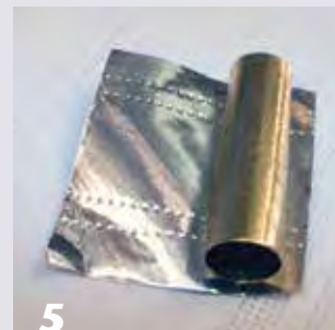
Peel the backing off the duct tape and adhere the base layer to the brass pen tubes.
